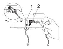
3. Thread the AC Power Cord through the clip on the base stand, and place the Base Unit on the desk or table top.
